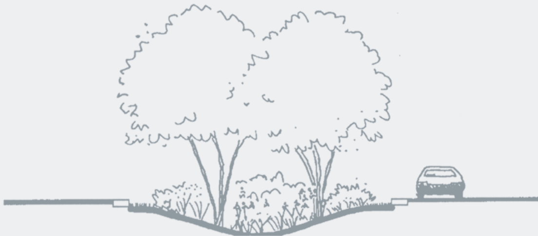
Cul-de-sac infiltration island accepts stormwater from surrounding pavement. Note flat curb.
